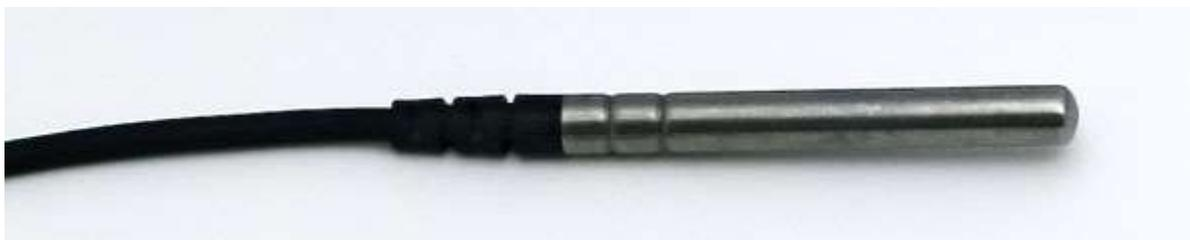
Rugged stainless steel probe 6 mm (0.236") diameter and 50 mm (approx 2 inch) length with 6.1 meter (20 ft) cable. TPE jacketed cable has diameter of 3.3 mm (0.13"), round cross section and 24 gage, polypropylene insulated leads. Suitable for immersion, HVAC, and soil burial applications. Probe's cable not recommended for immersion in fuels (fuel splashing on cable is OK).
