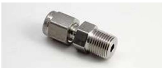
Bored-through stainless steel compression fitting for PT916 probe. 1/8 NPT male threads. 1.2 inches in length (30.5 mm).
