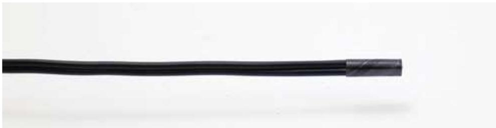
Epoxy tip with parallel 24 gage, PVC insulated leads (parallel bonded). For general purpose temperature measurement. Not for continuous immersion in water (mineral or silicon oil is OK).
